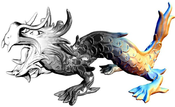
Figure 1: Dragon SLIM model rendered with our system with different shaders applied at roughly 40 fps. From left to right : NPR shading, Reflection mapping, Phong Shading.
