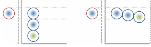
Figure 4. Self-occlusion handling. Inside boxes: Top view of 3D model SoG. Left of dotted line: Image plane with 2D Gaussian. Left column: As long as no occlusions happen, Eq. (5) calculates a correct overlap of a single element. In this example, the color (blue) and the shape are identical, yielding the similarity E_{ii} . Right column: If several 3D model Gaussians project to the same screen space coordinate, their contribution is cumulative, yielding a similarity larger than E_{ii} , even though two of the model Gaussians should be occluded. Using Eq. (8) correctly limits the contribution of a single 2D image Gaussian, yielding the same similarity E_{ii} for both cases.
